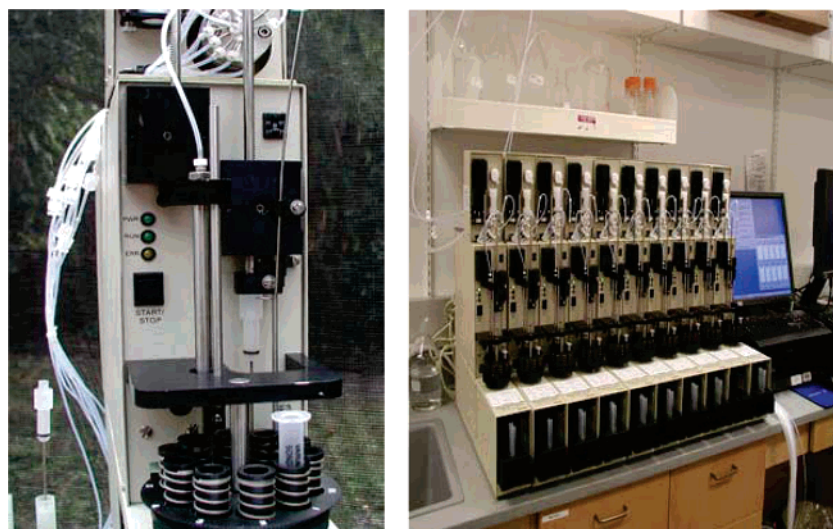
Figure 1. RapidTrace SPE workstation. (left, single modular unit for 10 cartridges; right, 10 units controlled by a PC).
